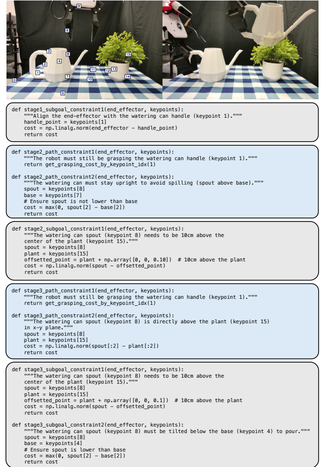
Figure 13. ReKep’s output for the pouring task and the resulting robot execution (top-right). The VLM predicts to grasp at keypoint 1, move keypoint 8 above 15 and 7 during transport, and above 15 and 4 for pouring—leading to failed execution.
